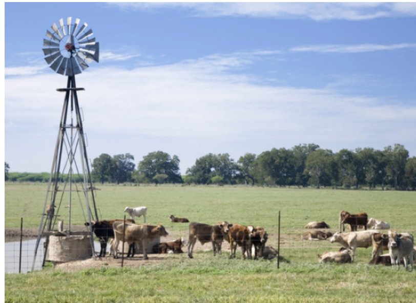
Figure 8.7 – Farm windmill used for pumping water
